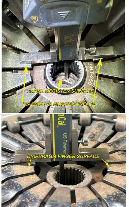
SOME CLUTCH / FLYWHEEL COMBINATIONS MAY NOT CONFORM TO THE NISSAN FACTORY STACK-UP DISTANCE WHICH CAN CAUSE DAMAGE TO THE C.S.C. IF NOT CORRECTED. CHECK THIS MEASUREMENT IF YOUR CLUTCH / FLYWHEEL COMBINATION ARE NOT KNOWN TO BE WITHIN FACTORY SPEC. ALL JWT AND OEM CLUTCH / FLYWHEELS ARE WITHIN SPECIFICATION.
